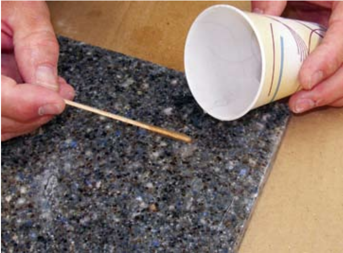
Figure Eight: Apply minimal amount of gel coat over patch, slightly over lapping existing gel coat.
